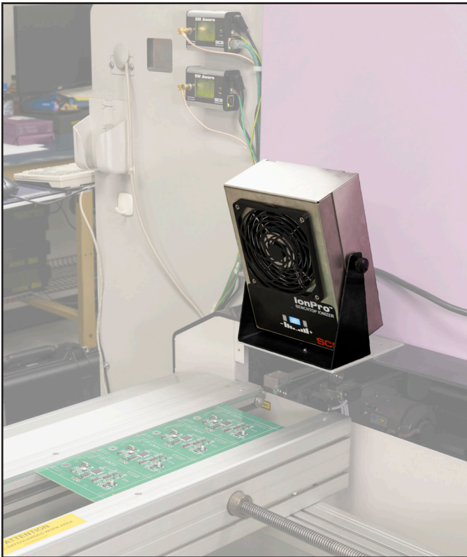
Figure 5. Using the Ion Pro™ Benchtop Ionizer at a machine station
